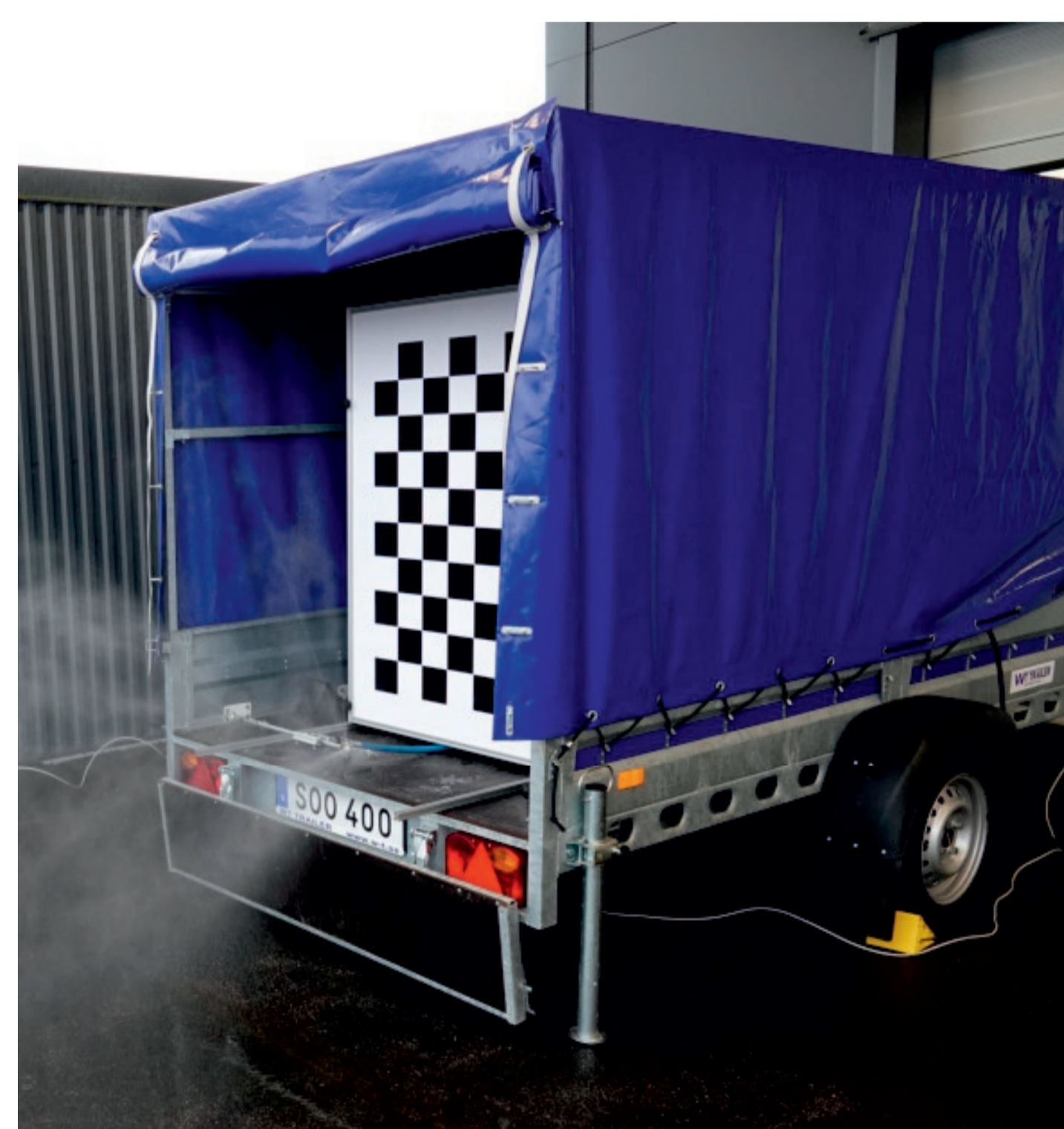
The AstaZero spray rig with a contrast board as the sensor target.
