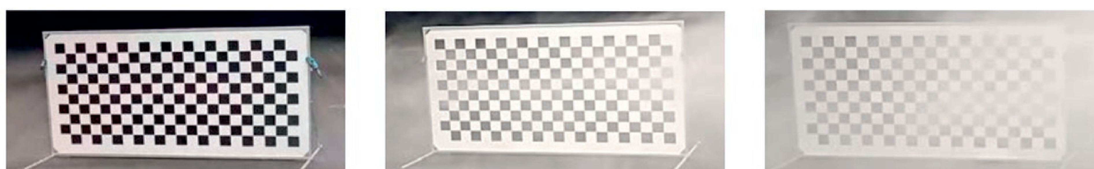
Contrast Attenuation (CA) adjustable from none to near 100% is possible. Pictures showing around 0, 20 and 70% CA
