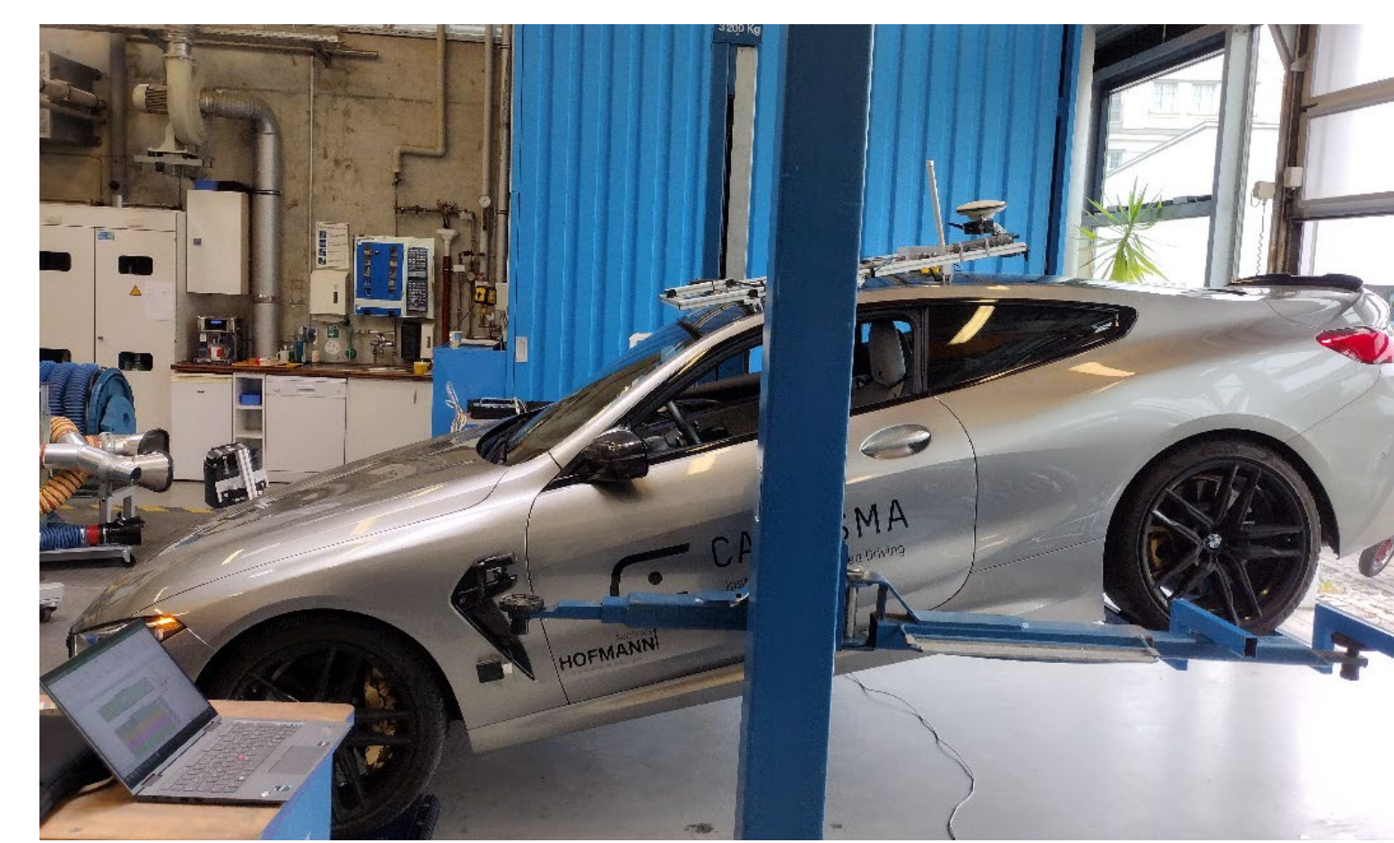
Figure 3. Measurement of CG position at C-IAD.
