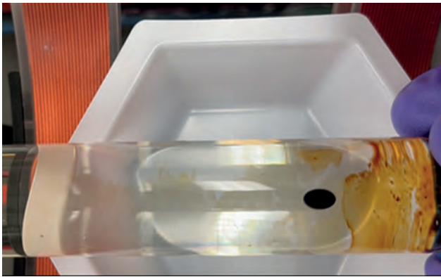
Elongation of a ferrofluid droplet in a quasi-uniform magnetic field (Helmholtz coil).
