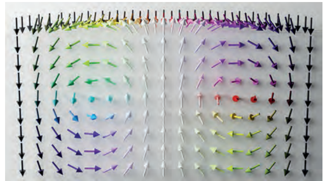
Fig. 1. The cross-sectional meron texture of a Bloch skyrmion with Néel caps.
