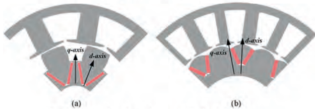
Fig. 2. Cross section of partial rotor. (a) 10s-8p, (b) 20s-18p.
