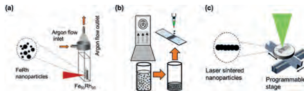
Fig. 1: Step-by-step pathway for producing magnetocaloric microstructure by a) Synthesis of FeRh nanoparticles then b) ink formulation and dispersion on glass substrate, and c) Sintering of FeRh dispersed ink.
