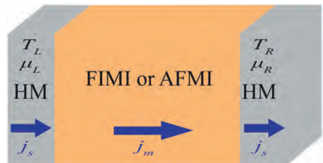
Schematic diagram that illustrates the transport of magnon current through FIMI or AFMI driven by temperature or spin chemical potential difference.
