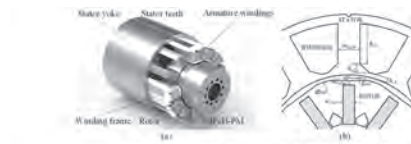
Fig. 3. Three-dimensional structure drawing and design parameters of the motor
