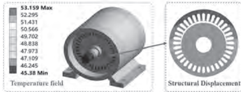
Fig.1 Temperature field and structural displacement result
