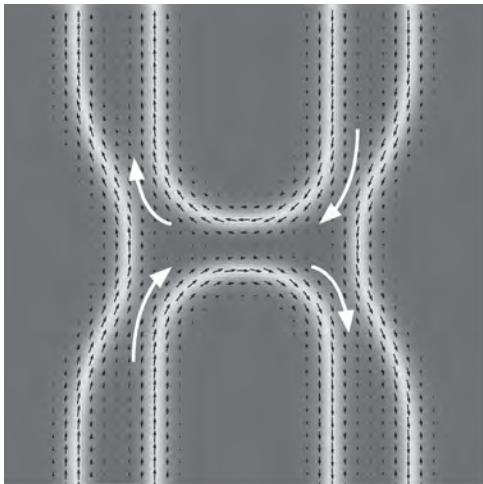
H stripe structure magnetization. Red/blue is out/into the plane. White arrows indicate DW chirality.
