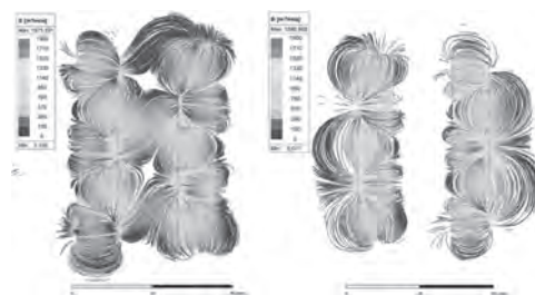
Flux diagram pointing for grasping (left) and dropping (right)
