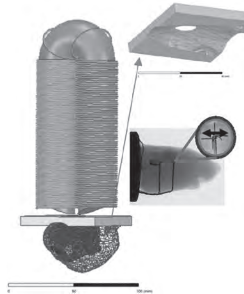
Fig. 1 Novel Parabolic Ferromagnetic Core (PFC) TMS coil with highly diamagnetic pyrolytic graphite shielding plate for a focused stimulation of the primary motor cortex (M1) of a rat's brain.
