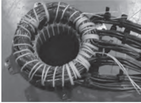
Fig.2. the armature of FLW star-delta connection
