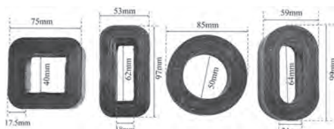
Fig. 1. Nanocrystalline cores and their sizes.
