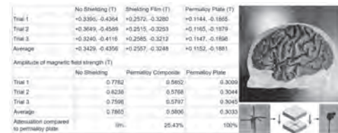
Fig. 2: TMS coil magnetic field strength with different shielding, brain phantom and dipole probe fabrication.
