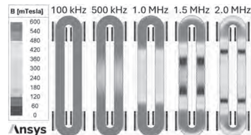
Fig. 1: Horizontal slice through the middle of the core's thickness
