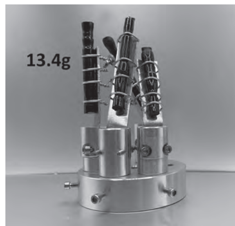
Fig.1. Single-crystal (13.4g) mount of Co_2SiO_4 , co-aligned in (hk0) -scattering plane
