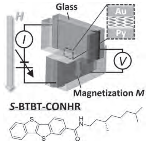
Fig. 1 Schematic of Au/ S -BTBT-CONHR/Py devices.
