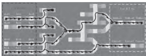
Figure 2. Micromagnetic simulation of pipelined full adder. Skyrmions are pipelined into the full adder form the left, encoding inputs ( A_0=0, B_0=1; A_0=0, B_0=1; A_1=1, B_2=1; A_3=1, B_3=0 ). Black lines represent their trajectories, and skyrmions are propagated according to the respective VCMA regions (light red/green/blue) using the VCMA waveform shown in Fig. 1(c). At t=0 ns (blue), the skyrmions are initialized and propagated rightward to the correct logical outputs at t=8.7 ns (green).
