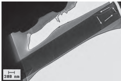
Fig. 1. Elongated domain wall in a highly magnetostrictive Fe-Si-B sample (LTEM).
