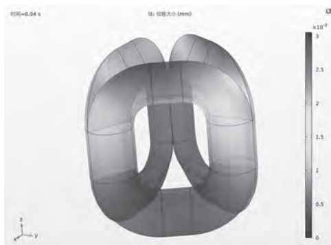
Fig. 2: Distribution of vibration displacement on core surface
