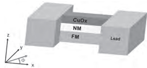
Fig.1(a) Schematic of Co/Pt/CuOx nanowire
