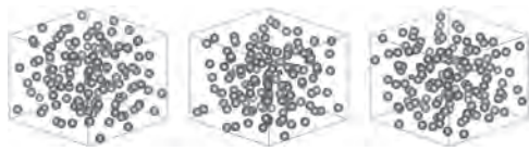
Fig. 1. Amorphous 100-atom cuboid cell: (a) \text{Fe}_{80}\text{P}_{13}\text{C}_7 , (b) \text{Fe}_{80}\text{P}_{11}\text{C}_7\text{Ge}_2 , and (c) \text{Fe}_{80}\text{P}_9\text{C}_7\text{Ge}_4
