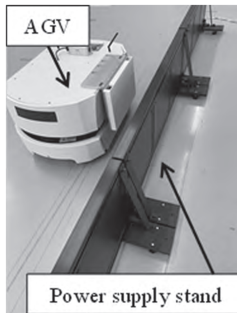
Fig. 1. Image of power supply to operating AGV
